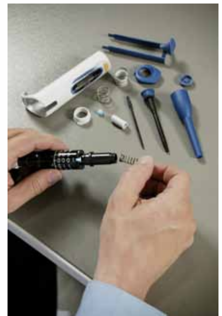
Pipettes are dismantled, cleaned and new parts fitted where necessary
