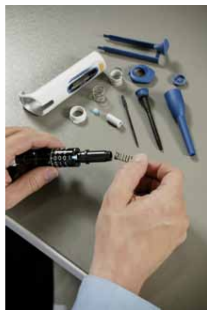
Pipettes are dismantled, cleaned and new parts fitted where necessary
