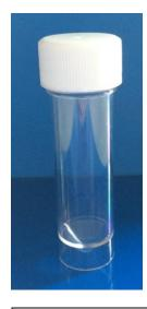
30ml Universal container in clear polystyrene with a high density polyethylene screw cap with integral low density expanded polyethylene seal.
