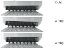
Briefly press the Decap button (green) to initiate tube opening. While decapping, move the Decapper upwards (away from tubes).
