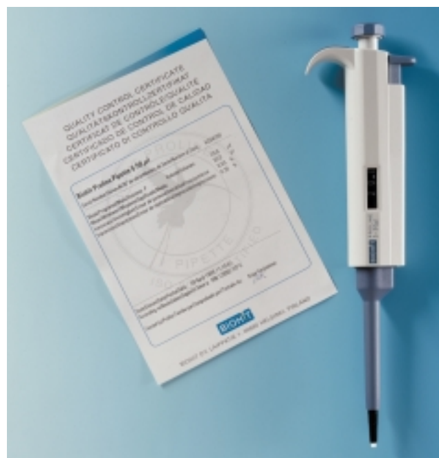
Fig. 2. Each individual pipettor receives a QC-certificate, where most often the performance testing is done according to DIN 12650.
