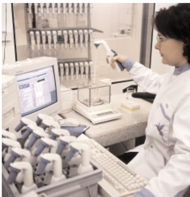
Fig. 1. Performance checking of a pipettor using the gravimetric method monitored by a computer.
